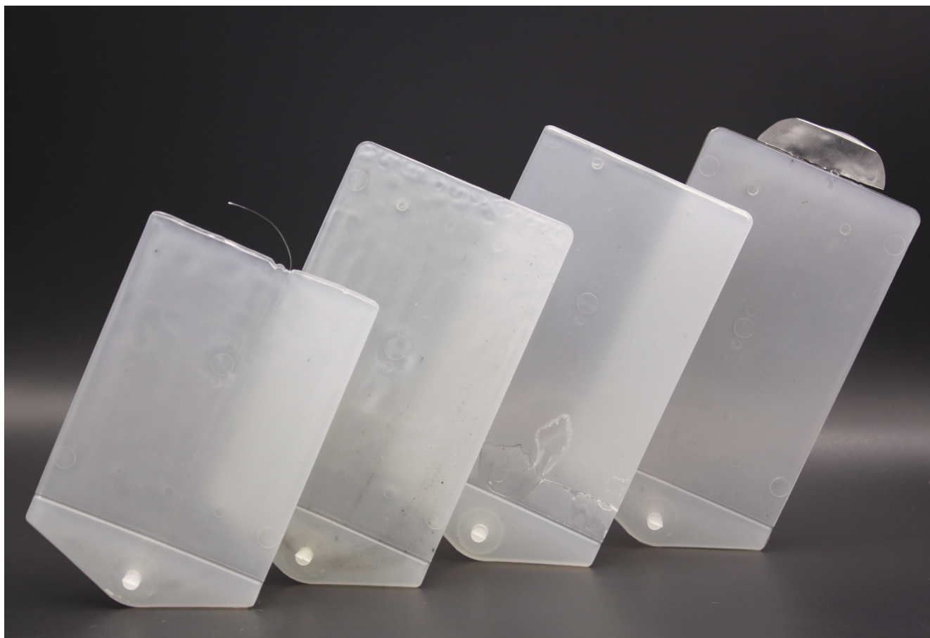
Typical injection molding defects, caused by incorrect switchover from injection to holding pressure phase (© IKV)
