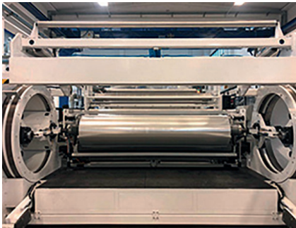
The system consists of a multi-roller cast unit with two separate cast zones, which allows getting the right set-up in order to cover a very wide thickness range, from flexible film to foil (© Colines)
